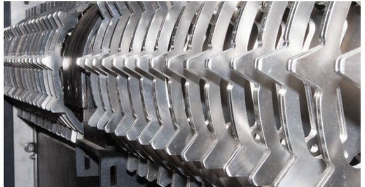
Full-width, chainless positive drive system reduces risk of catastrophic failure.
