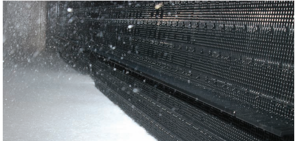
The spray bar cleans away debris on the working Series 6000 screen.
